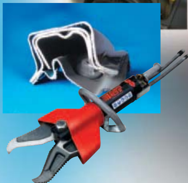
figure 2: The bar in the crushable zone can be made of micro-alloy steel or Boron steel.
