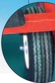
Pneumatic tyres to prevent walking of the fan. Tyres are fitted at the back to allow walking on stairs without damage and absorb the vibration of the fan.
